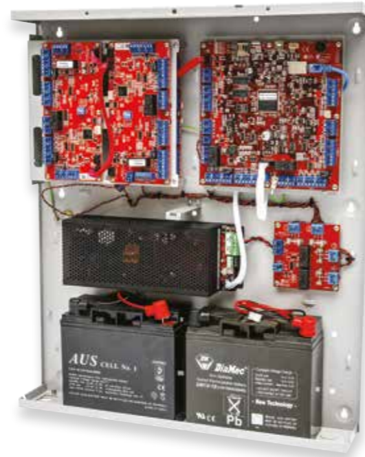
ABOVE: IAC shown in 8 Door / 10 Reader configuration. (IAC with UniBus 2 Door / 2 Reader expansion devices connected). Housed in the WideBody enclosure with hinge plate, 8Amp PSU, Fire Door override relay card and 2x 17Ah batteries
