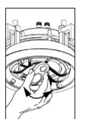
Figure 4. Midrange/tweeter pod adjustment
